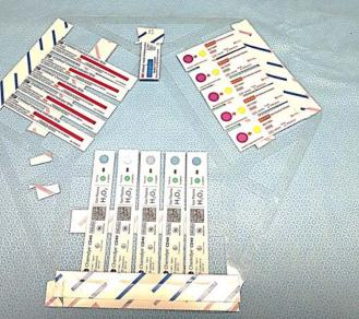
Mounted on a pre cut acetate sample holder using vH2O2 indicator tape
