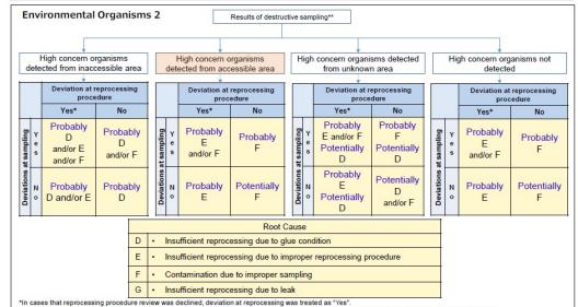
\*\* In case leak was detected during destructive sampling, root cause "G" was added as probable cause in addition to the determination on the table above
